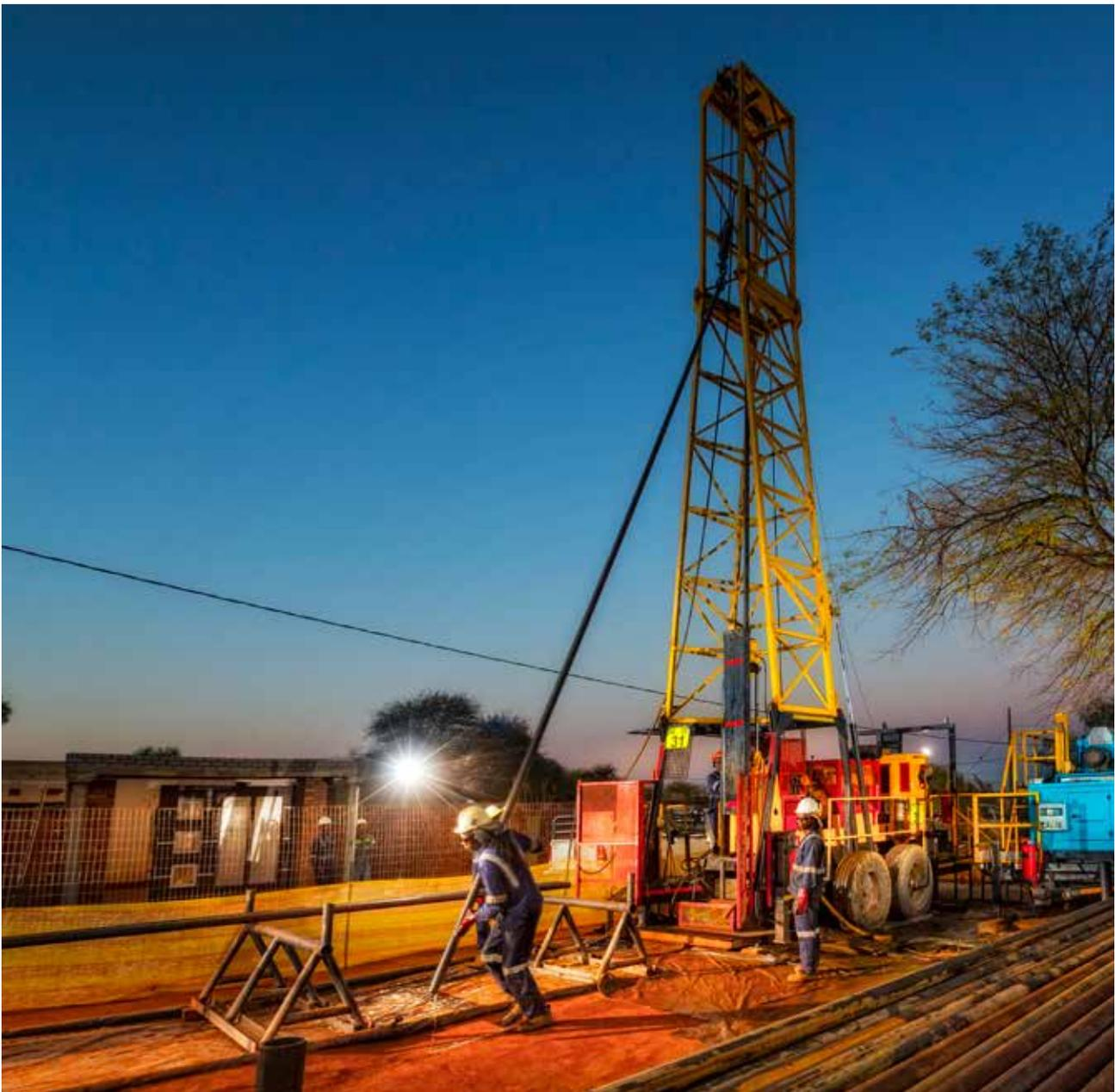
Exploration drilling, BRPM North shaft Phase III investment area
