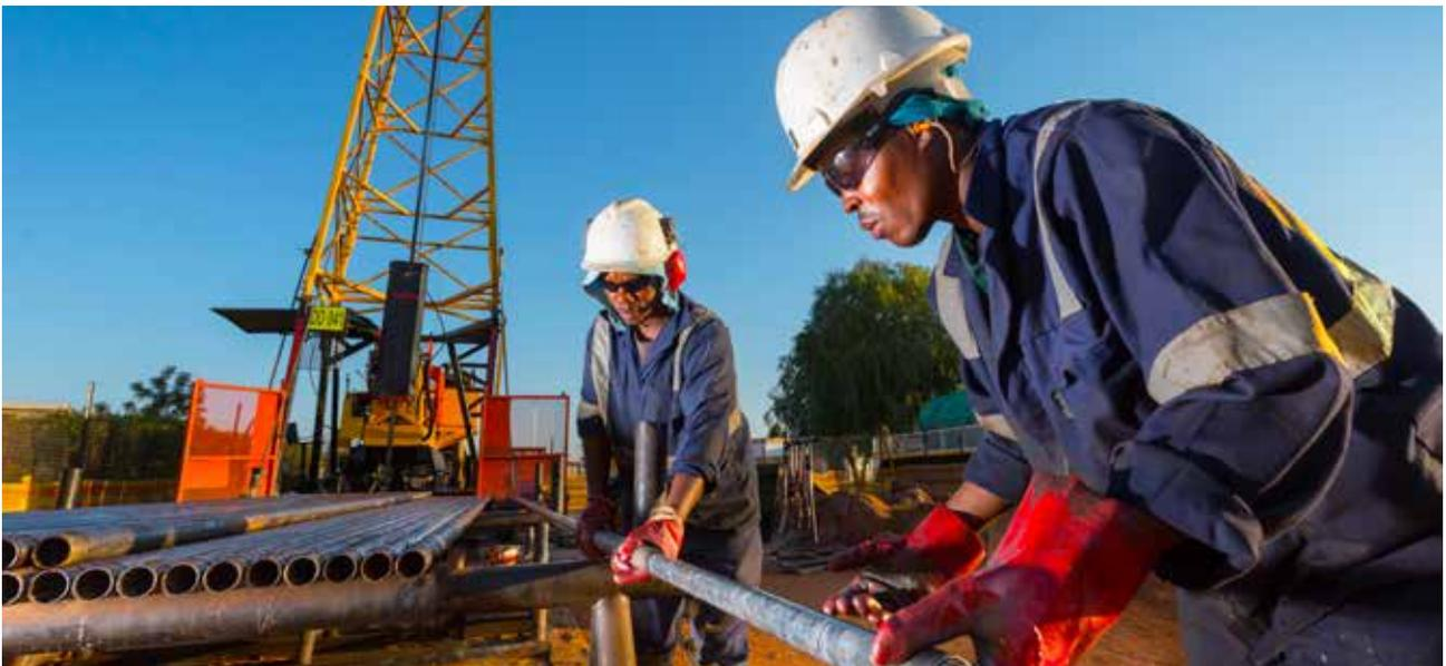
Exploration drilling core extraction, BRPM North shaft Phase III investment area
