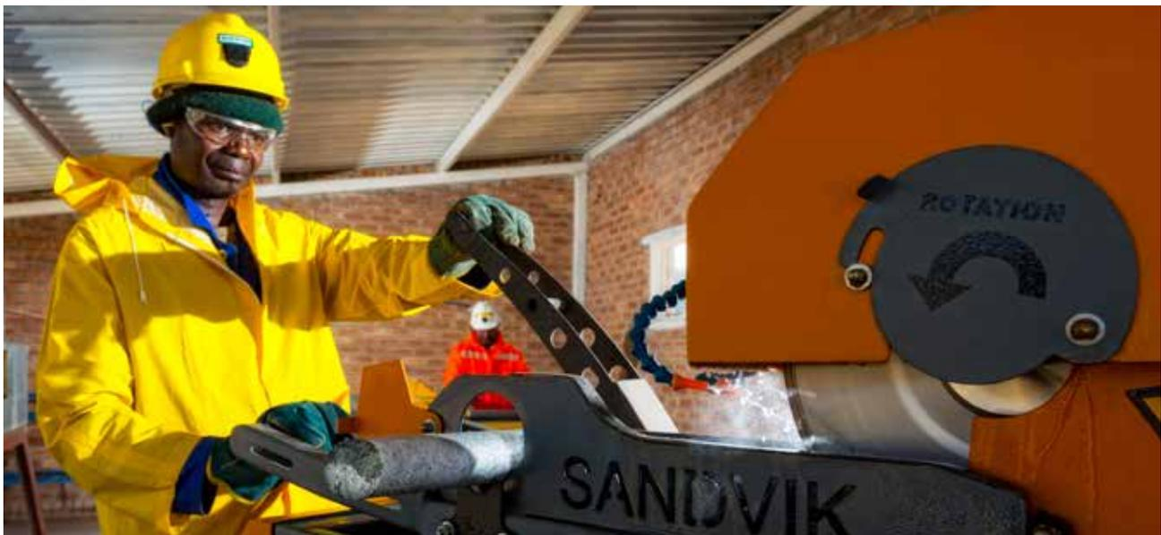
Exploration drillcore sampling, RBPlat exploration coreyard
