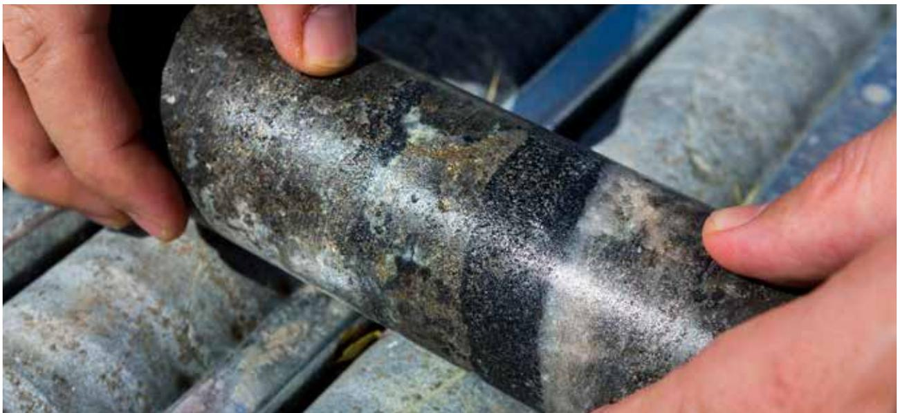
Surface exploration drillcore, Merensky Reef intersection Styldrift I shaft area
