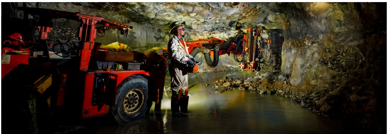
Mechanised roof bolt installation on 600 Level at Styldrift
