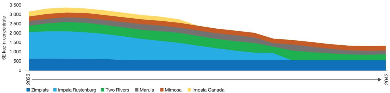
The pictorial 20-year profile in this chapter is shown below as a combination of level I with selected level IA, II and III profiles. Only LoM I is based on Mineral Reserves, while LoM II and III have not been converted to Mineral Reserves. Therefore, this combined graph shows a similar low profile from 2036 onwards compared to the profile published on 30 June 2021.
