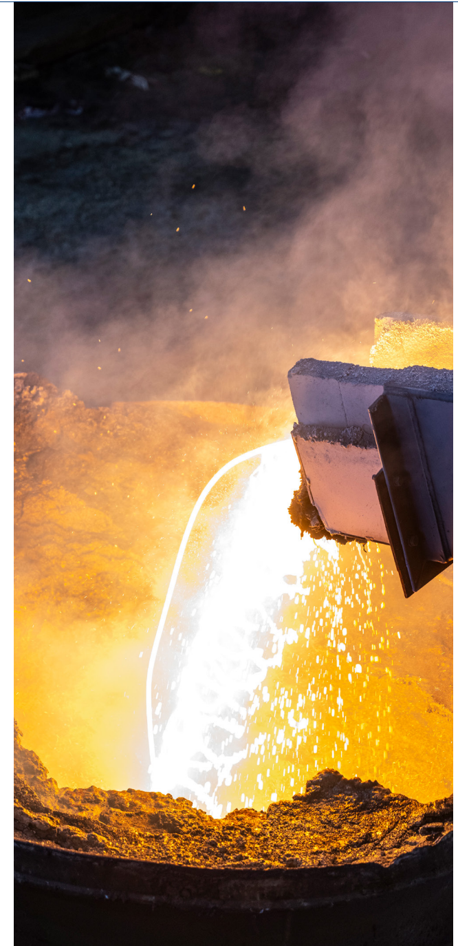
Lancing one of the furnaces with an oxygen lance at Impala Rustenburg
