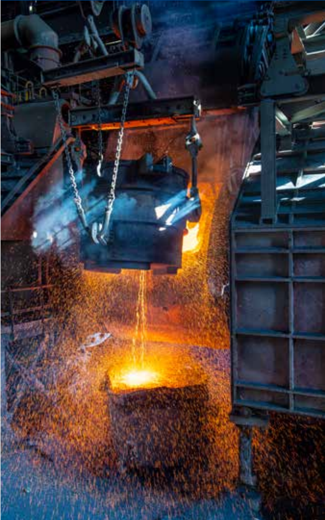
Ladle transfer of molten furnace matte to a converter
